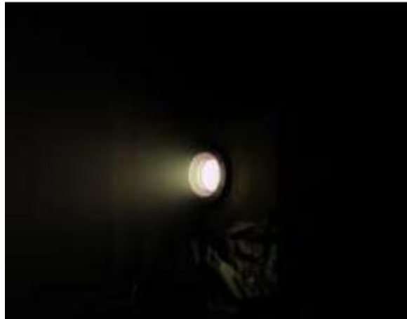
Figure 14. RIT-10 operating on a nitrogen/oxygen mixture [54].
